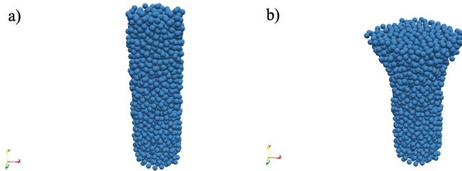
**Fig. 1.** Test of deformation in dynamic compression of aluminum sample. Initial geometry a) and deformed sample b).
