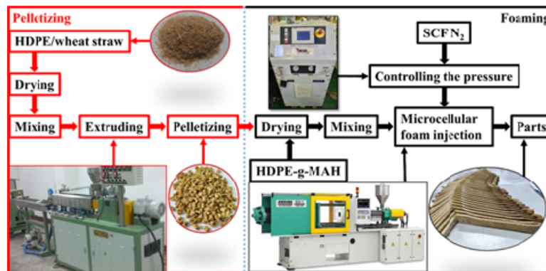
Fig. 1. The flow chart of microcellular injection molding process.
