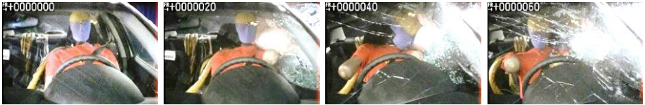
Fig. 1. Occupant's impact by side structure of the vehicle body deforming during the front-to-side cars crash test; frames every 0.02 s from the beginning of the collision contact [3]
