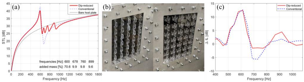
Fig. 1. (a) Predicted STL of conventional and optimized dip-reduced metamaterial panel with its parameters, (b) manufactured conventional (left) and dip-reduced (right) metamaterial panels mounted on the acoustic testing cabin and (c) comparison of the \Delta IL of the conventional and dip-reduced metamaterial panel in 1/12 octave bands.
